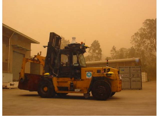
Figure 1: The autonomous Hot Metal Carrier undertaking payload handling operations in a duststorm.
