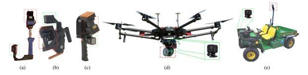
Fig. 1: Examples of mobile mapping devices with various lidar configurations, ranging from handheld (a-c), to aerial (d) and ground (e) platforms. The original lidar device is highlighted in red, while the added camera (which is not connected or synchronised to the lidar) is indicated by the green box. References for the lidar mapping devices: (a) Zebedee [2], (b) CSIRO Revo, (c) ZebCam [5], (d) Hovermap [6], (e) Gator [7].
