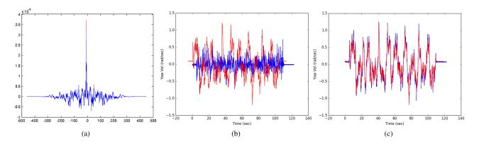
Fig. 3: Examples of (a) the cross-correlation output, (b) poor time synchronisation, (c) successful time synchronisation. The red and blue signals represent the yaw-rates of the camera and lidar, respectively.
