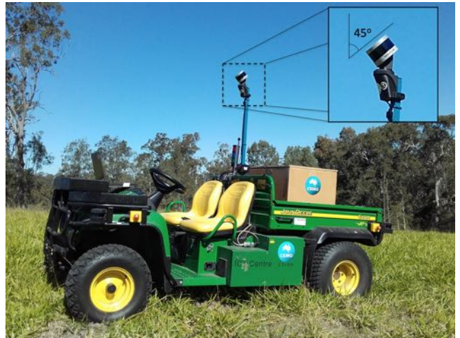
Fig. 7: The John Deere Gator platform automated by the CSIRO. The LiDAR Velodyne sensor is mounted above the vehicle and is rotated by a motor at a 45^\circ angle.
