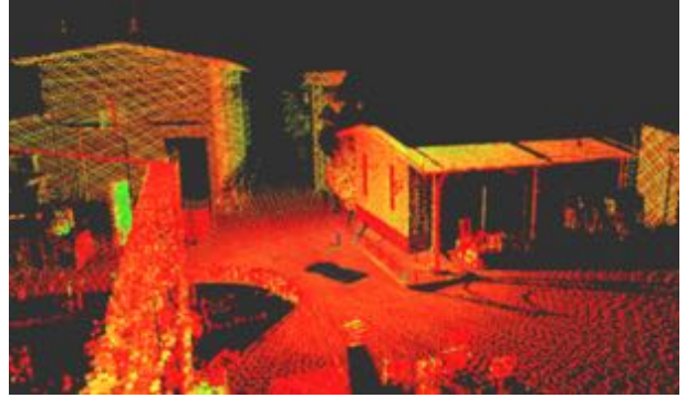
(b) Corresponding intensity coloured point cloud as scanned from the vehicle.
