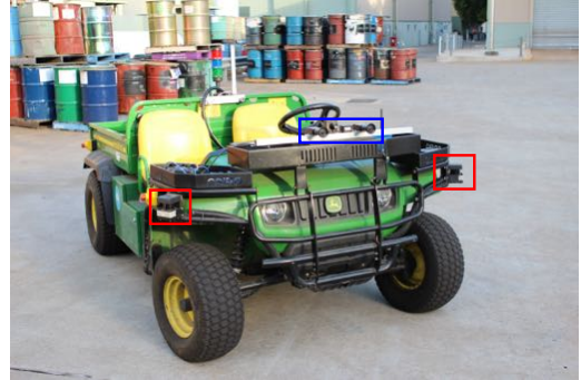
Fig. 5. The test vehicle, a John Deere Gator holding multiple sensors of which the two laser range finders (red boxes) and the stereo vision sensor (blue box) were used.
