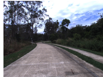
(b) This region has a road delimited by grass. A laser set-up can not detect the grass as a non-traversable area.
