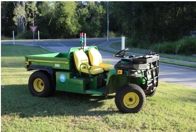
Figure 4: The test vehicle, a John Deere Gator holding multiple sensors (lasers, camera, wheel odometry) was used.
