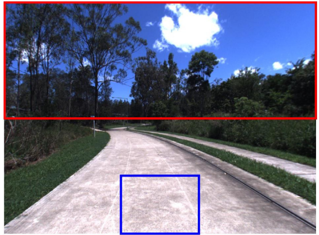
Figure 7: This image shows the auto-labelling procedure. Pixels taken from the red rectangle were labelled as background while pixels taken from the blue rectangle were labelled as road.
