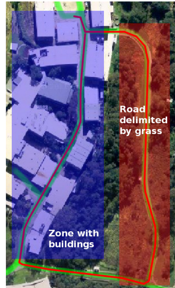
(a) The trajectory to be followed is marked in red. Similarly, different regions where the sensors may not perform correctly are highlighted.
