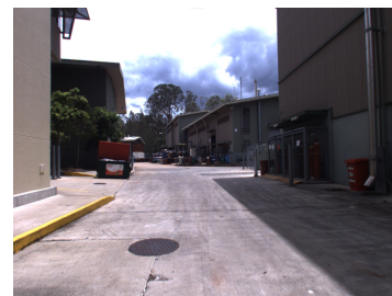
(c) The colour of the sidewalk and buildings in this section may cause false positives in the visual road-detection algorithm. Similarly, the strong shadows also affect the outcome of the algorithm.
