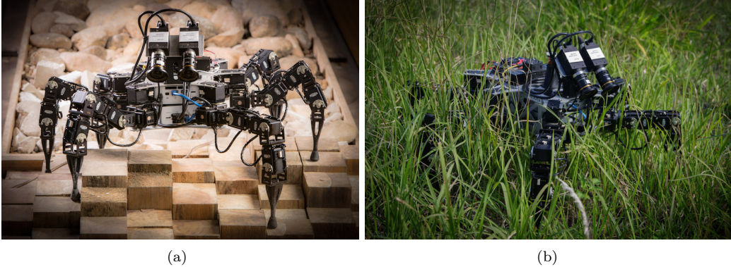
Figure 1: Hexapod robot Weaver on (a) the multi-terrain testbed and (b) outdoor terrain.
