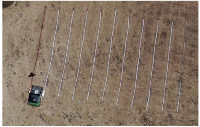
Figure 10: The result of scanning 10 rows of an area representing a minefield, by line following each painted lane in turn.
