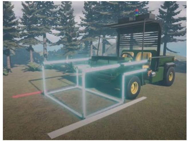
Figure 2: Illustration of the low-resolution magnetic sensor (highlighted in white) that can be mounted on the vehicle.
