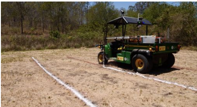
Figure 9: Illustration of the ‘live’ spraying of white paint over red paint. The small precision errors shown in Table 2 do not affect the practical performance of the marking system.
