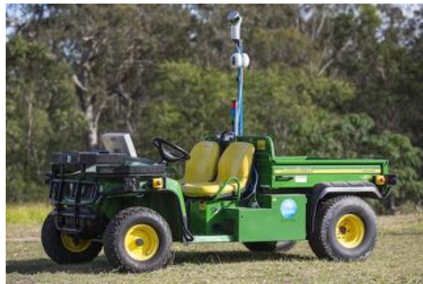
Fig. 4. Robotic platform used for testing is an automated John Deere Gator at the CSIRO's QCAT research facility.
