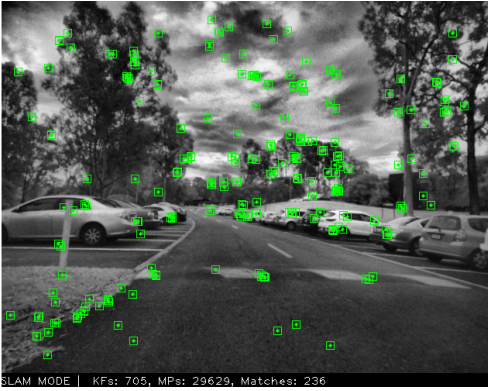
Fig. 5: Sample image after the Adaptive Histogram Equalization, the green dots stands for the detected ORB features.
