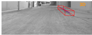
(b) Gamma-corrected lower half of the left image. A line detected by the Hough transform (blue) is projected into the image and the test box around it is indicated in red.
