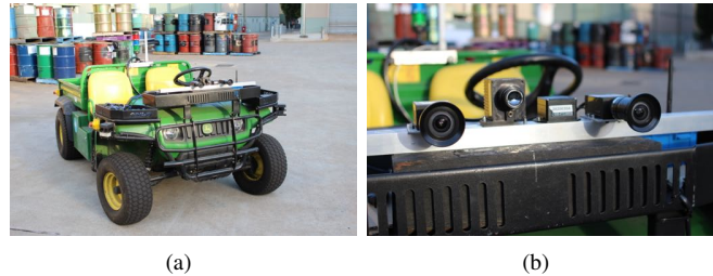
Fig. 6. (a): John Deere's Gator, the test vehicle used for the experiments. (b): The point Grey Grasshopper cameras mounted on their stereo rig, approximately 1 meter above the ground. Obs.: The thermal camera and the inertial measurement unit in the center of the rig were not used in this work.
