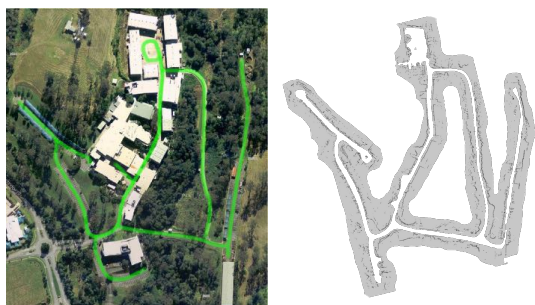
(a) Satellite view of the test area (the drivable routes are highlighted in green), illustrating the structured and un-structured routes. The scale is 410 \times 360 meters. (b) Map of the test area from vehicle. The laser-based localizing structured and un-structured routes. The scale is 410 \times 360 meters.
