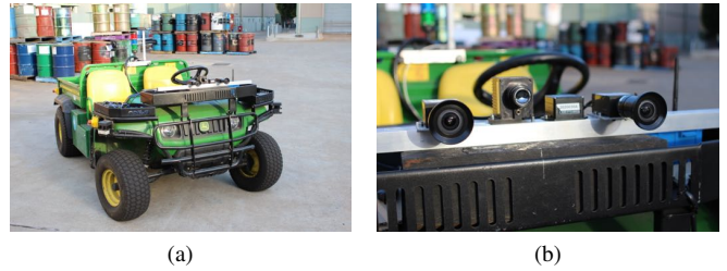
Fig. 12. (a): John Deere's Gator, the test vehicle used for the experiments. (b): The point Grey Grasshopper cameras mounted on their stereo rig, approximately 1 meter above the ground. Obs.: The thermal camera and the inertial measurement unit in the center of the rig were not used in this work.
